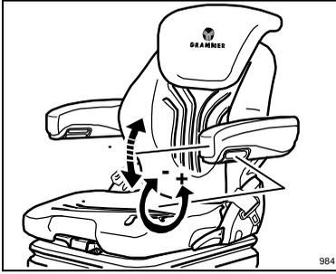
The inclination of the armrests can be modified by turning the adjustment knob.
